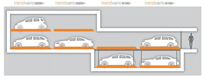
All TrendVario-plus models can be combined any way you like, one after the other, in up to 4 rows. The "plus" stands for the model that can be driven on.
