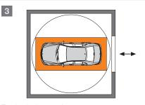
Turning in the transfer compartment with turntable
