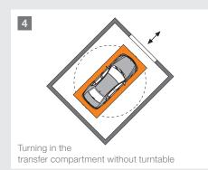
1 With one door: Drive in forwards, reverse out. 2 With two doors: Drive in forwards, drive out forwards. 3 With vehicle turntable and one door: Drive in forwards, drive out forwards. 4 Furthermore, driving in and out at various angles is possible.
