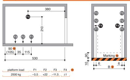
Units are dowelled to the floor. Drilling depth: approx. 15 cm.
