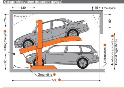
Before lowering the platform, the vehicle parked on the lower parking space must be driven off!
