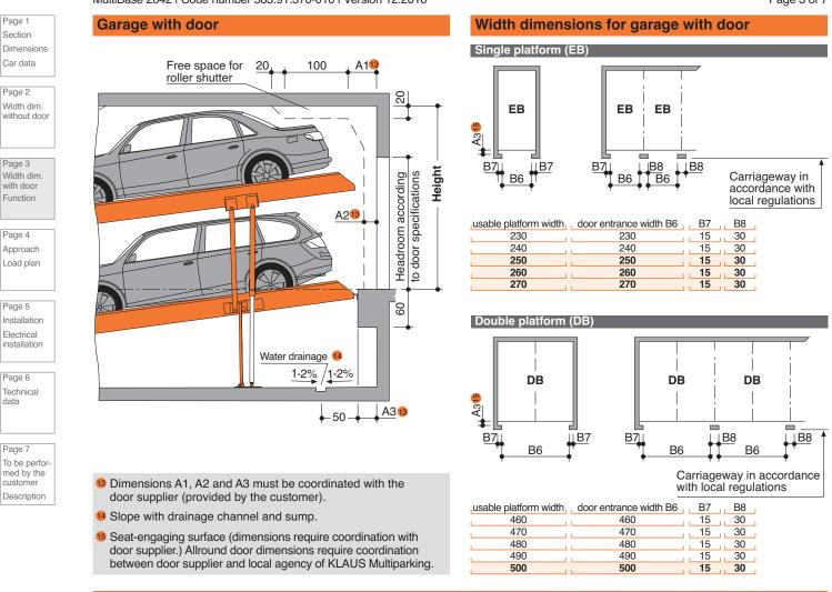
For parking boxes on the edges and boxes with intermediate walls we recommend our maximum platform width of 270 cm for single platforms and 500 for double platforms. Problems may occur if smaller platform widths are used (depending on car type, access and individual driving behaviour and capability).
