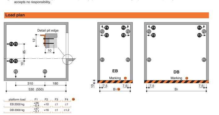
Units are dowelled to the floor. Drilling depth: approx. 15 cm.
