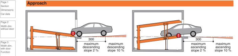
The illustrated maximum approach angles must not be exceeded. Incorrect approach angles will cause serious
